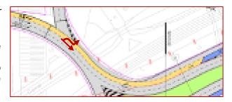
A bifurcation arrow has been indicated at the exit from the rotary, however this may be insufficient notice for drivers wishing to leave at the upcoming off-ramp, resulting in late lane-change manoeuvres and possible side-swipe collisions.
